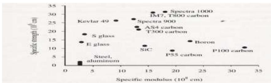
Fig 8 Specific Modulus And Specific Strength For Various Engineering Materials And Fibers (Swanson S.R; 1997; 3)
