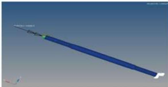
**Fig.10** Loading and boundary conditions on composite which drive shaft
